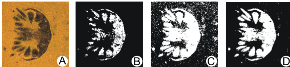
Fig. 3: Figure 3. Linear Generation examples. A; source image. B; too dark.(to few white pixels) C; too light (too many white pixels). D; about right.
